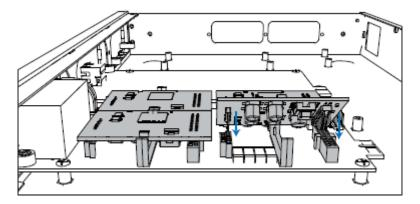
**STEP 6** Insert a SIM card on the GSM/CDMA/3G module following the instructions. Skip this step if no GSM/CDMA/3G module installed.
