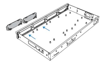
**STEP 2** Push out the empty board from the inside of the device.
