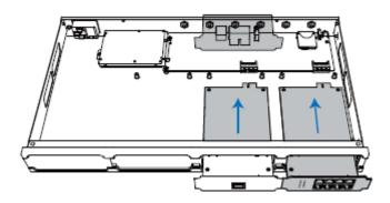
**STEP 4** Lock the screws to fix the Expansion Board.
