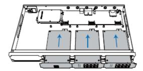
**STEP 4** Lock the screws to fix the Expansion Board.
