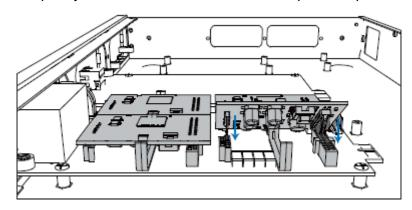
**STEP 6** Insert a SIM card on the GSM/CDMA/3G module following the instructions. Skip this step if no GSM/CDMA/3G module installed.
