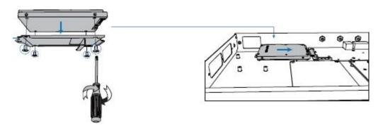
**STEP 2** Lock the screw to fix the hard disk.
